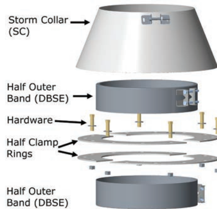
Figure 66a - Guy Section Details
