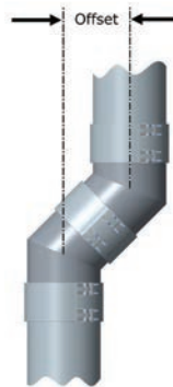
Figure 36a - Offset of two elbows
